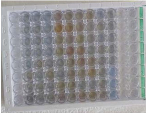
Figure 1. Appearance of the plate after adding the sample, antibody and Streptavidin HRP
